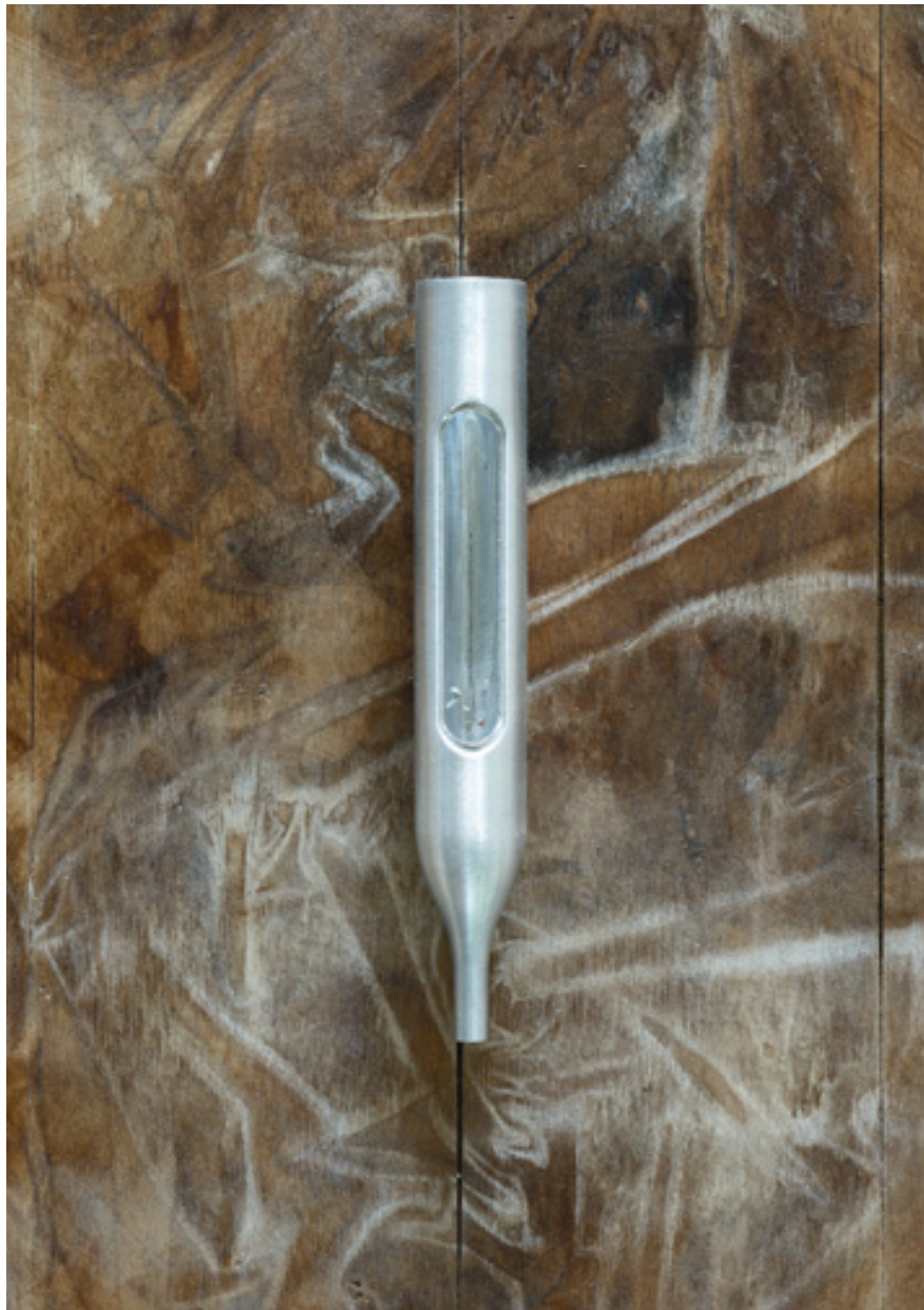
Flo head after finishing in the workshop. The next step will be painting or electroplating.
