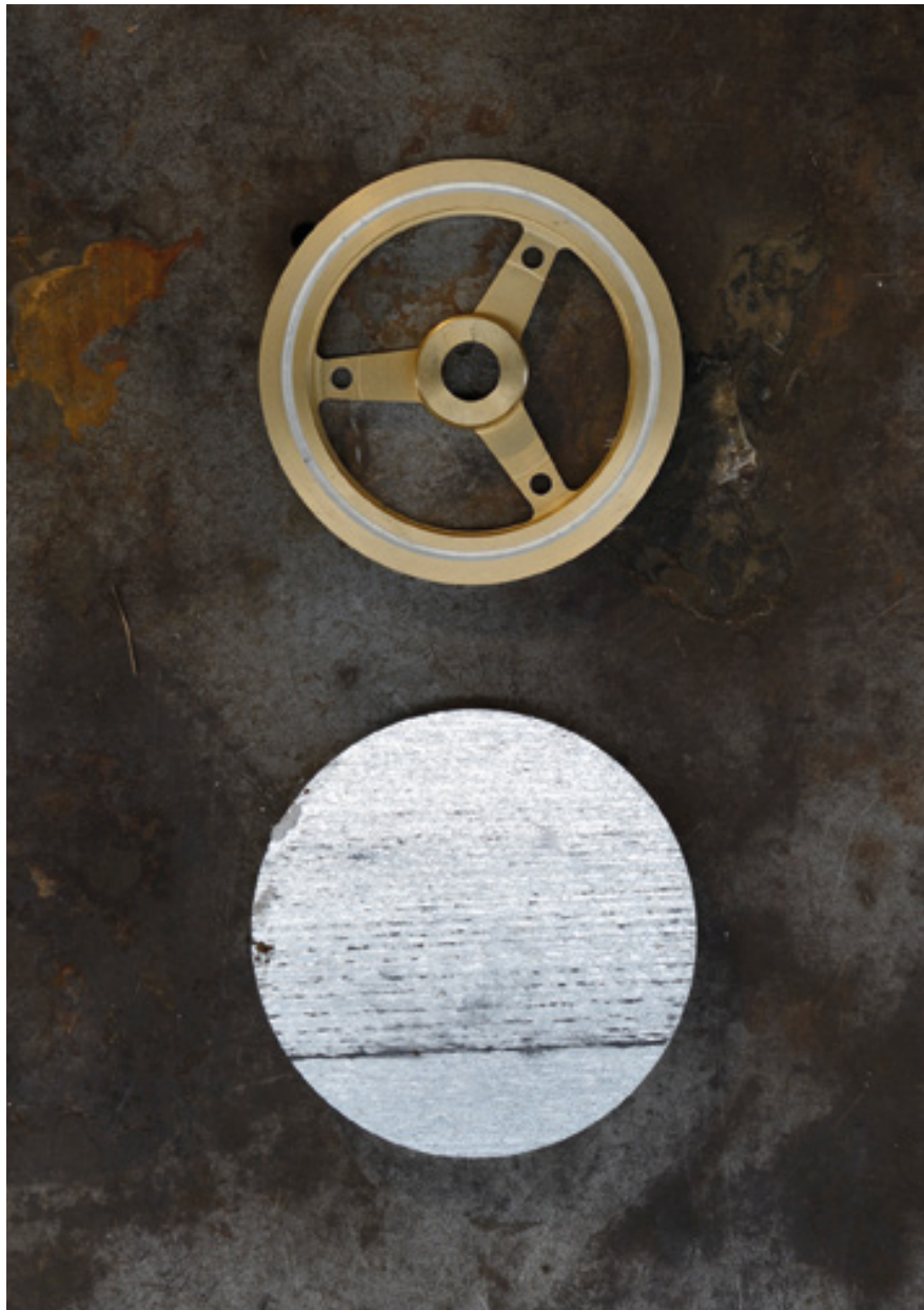
Top: finished, electroplated central wheel. Bottom: the unprocessed piece of aluminium from which it was made (on a CNC lathe).
