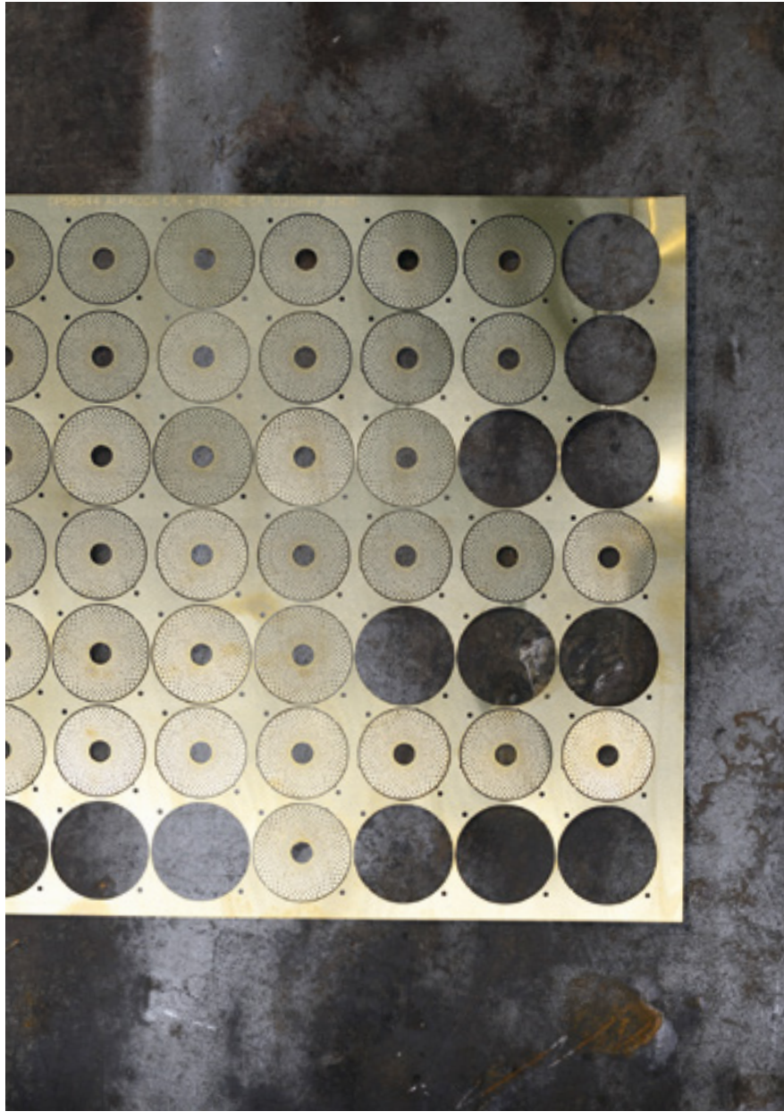
Chemically photoengraved brass sheet from which Tia's optical filters are extracted.
