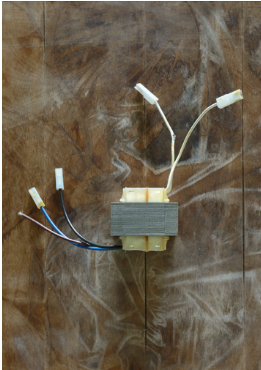
Double winding electromechanical transformer (50W/12V).
