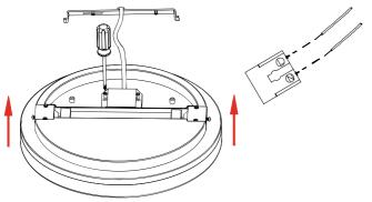
3. Wire "L" "N" to terminal block and mount ceiling light into the right place
